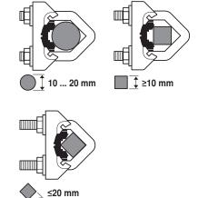
When using a round spindle made of CrNi (INOX):  $\varnothing$  12...20 mm
