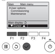
Press F1, F2 to move the cursor. Press  $(\checkmark)$  to go to the next screen.
