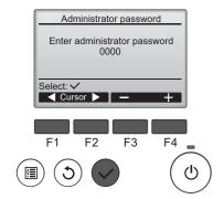
Press  $\boxed{F1}$ ,  $\boxed{F2}$  to move the cursor. Press  $\boxed{F3}$ ,  $\boxed{F4}$  to change the number. Press  $(\checkmark)$  to set the password.
