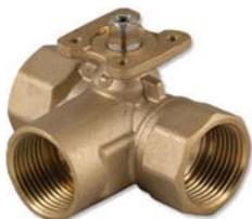
BV control ball valves are for regulating the flow of hot or cold water. They are controlled by a Lufberg DA actuator, which itself is controlled by a signal from the temperature regulator of the HVAC system.
