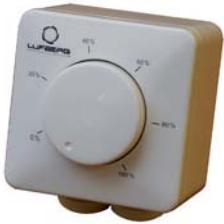
This potentiometer is designed to control actuators or EC-fans. It is mounted in a splash water proof design enclosure and can be used for inset as well as for surface mounting. It provides a proportional output signal between 0 - 10 VDC adjustable with internal trimmers: V1 and V2. The potentiometer has off-position.
