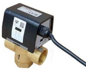
ZV-S zone valves are recommended for all heating and cooling systems with a required safety function for electrical supply interruption. In this case, the spring will safely close.
